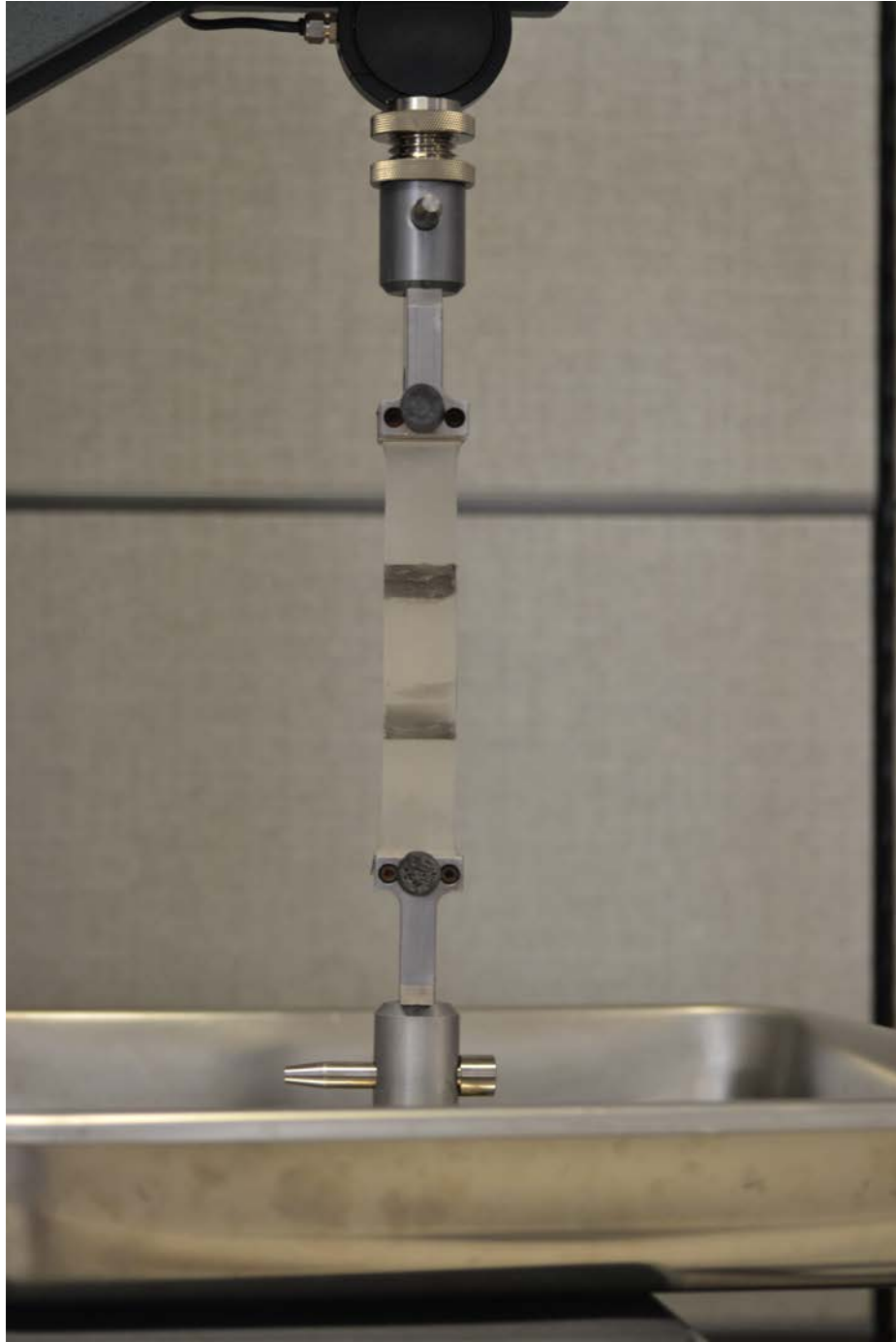
Figure 3.12: 4.8mm X 125mm X 21mm PDMS sample clamped into tensometer.
