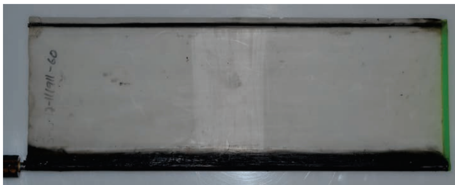
Figure 3.8: 112mm chord length flexible airfoil.
