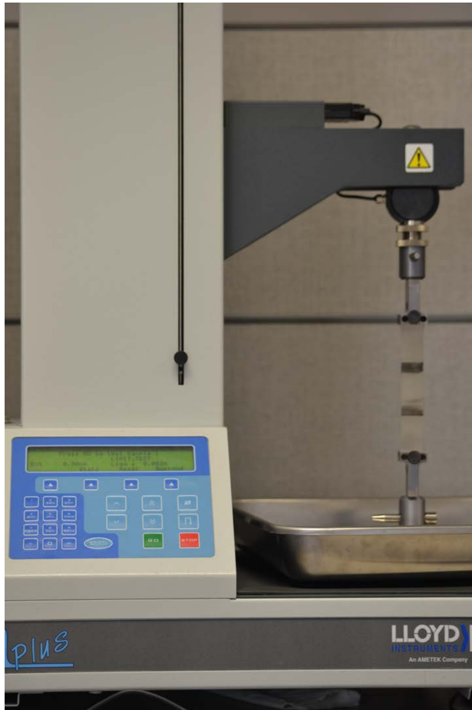
Figure 3.11: Lloyd Instrument LS1 Digital Material Tester with 4.8mm X 125mm X 21mm sample.
