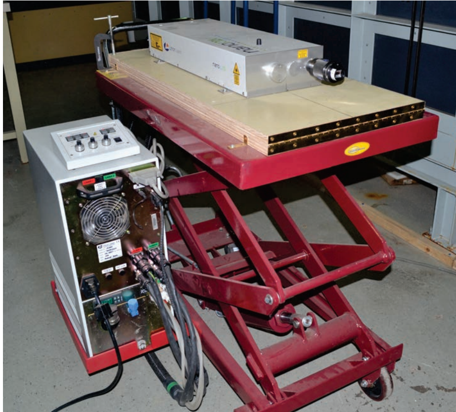
Figure 3.13: Nd:YAG Laser used for PIV.
