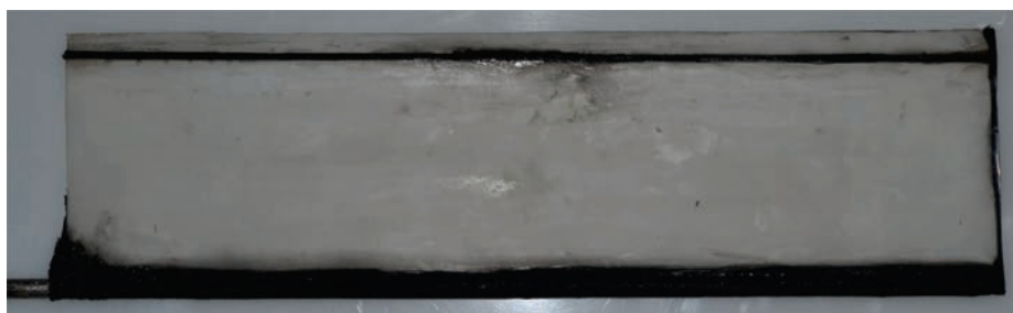
Figure 3.9: 82.55mm chord length flexible airfoil.
