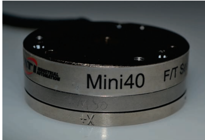
Figure 3.21: ATI Mini40-E Six-Axis Force Transducer.
