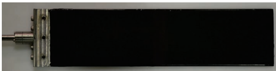
Figure 3.10: 76.2mm chord length rigid airfoil.
