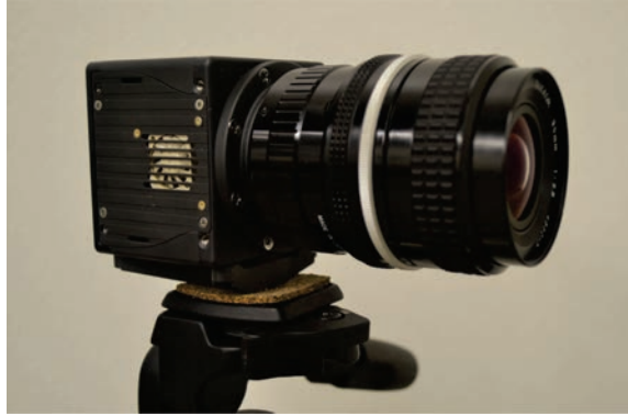
Figure 3.17: IDT NX4-S1 high speed camera.
